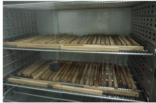
Figure 6. Conditioning teak wood after improvement with the microwave.
