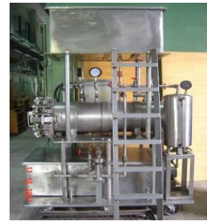
Wood impregnation vessel
